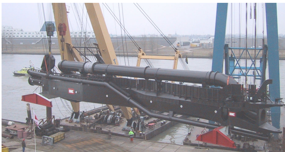
Fig 3. Lifting the upper pipe with submerged dredge pump unit of the Vasco Da Gama
